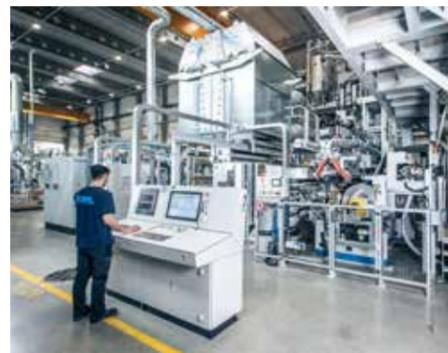
SML's FlexPack coating & laminating line
