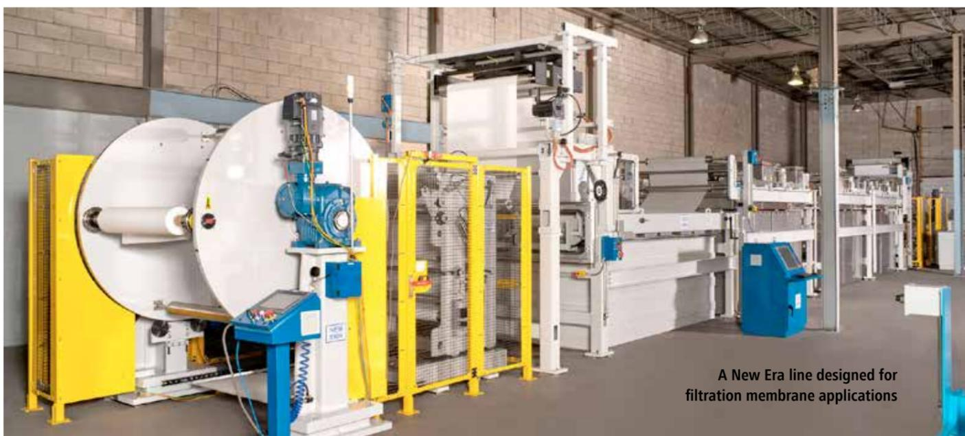
A New Era line designed for filtration membrane applications
