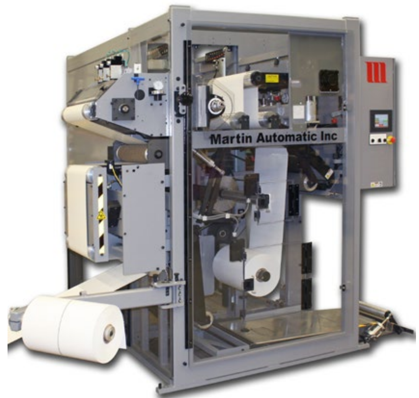
The LRD transfer rewriter with inline slitting has an optional articulating arm that automatically removes finished rolls through the side of the unit
